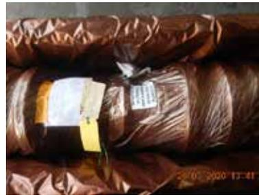
Macmahon's Southeast Asian operation, Batu Hijau, is supported by the company's workshop in Perth and uses local supplier R Moore & Sons to repair crankshafts and engine blocks. When returning the repaired parts to Indonesia, an anti-corrosion solution was required that would also allow for customs quarantine
